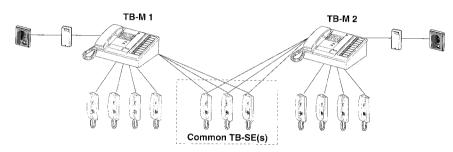
Two masters call and communicate with each assigned select button. Transfer of a sub's call to another on the other master is not possible.
